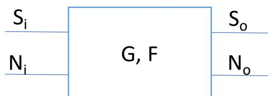
$$F(f) = \frac{\text{PSD of total noise at the output}}{\text{PSD at the output due to source resistance}} = \frac{N_o(f)}{G(f) \cdot N_i(f)}$$
