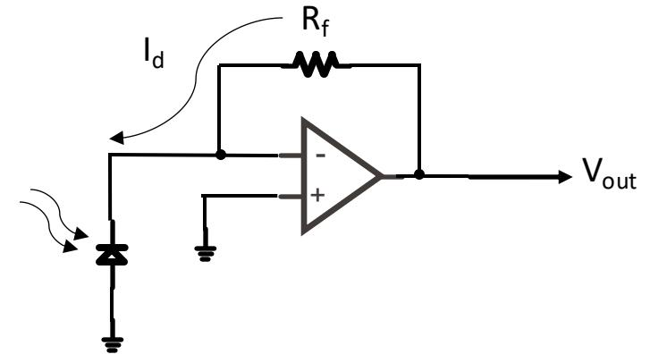
$$R_s = 50\Omega, C_L = 1 \text{ pF}, I_d = 20 \mu\text{A}, R_f = 5 \text{ k}\Omega$$
